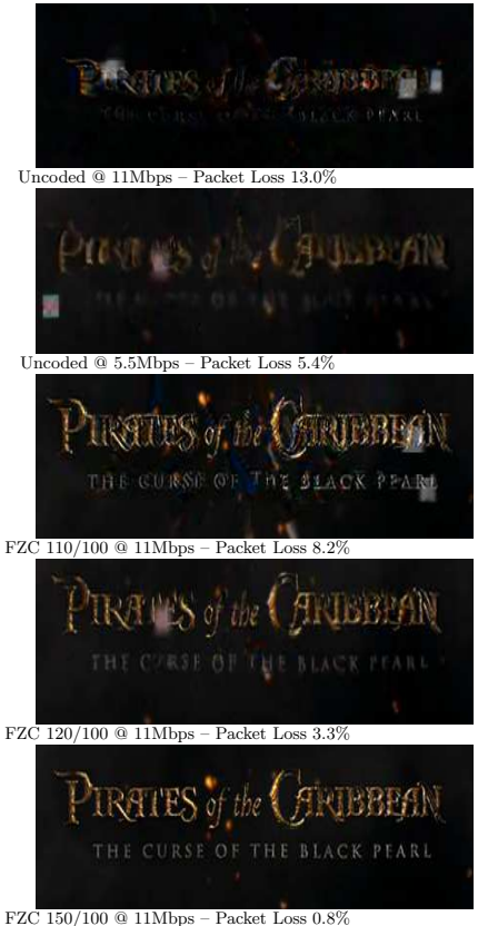
Fig. 2.23. Samples of the streamed video trailer at different coding and bit rates.
