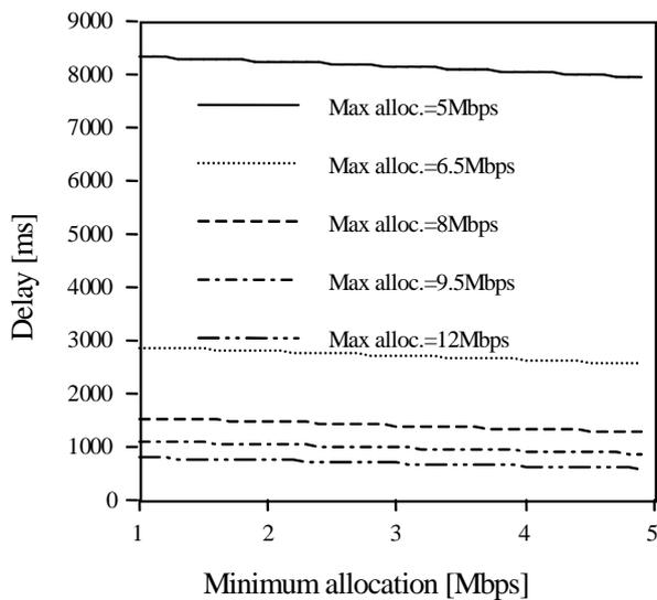
Figure 4: Maximum data delay vs. minimum allocation. 100 allocation levels with maximum allocations equal to 5, 6.5, 8, 9.5, and 12 Mbps.
