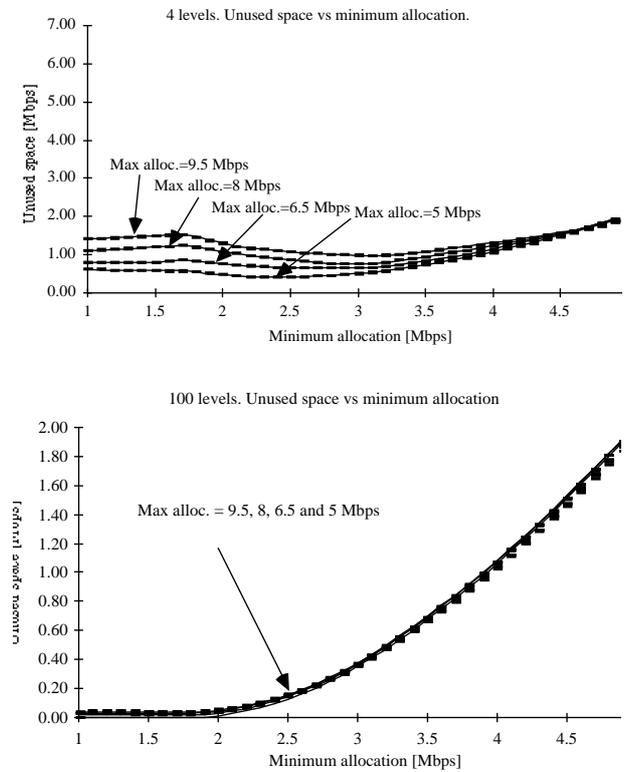
Figure 6. Four and hundred levels. Unused space vs. minimum allocation for various values of the maximum allocation with 95% confidence intervals.
