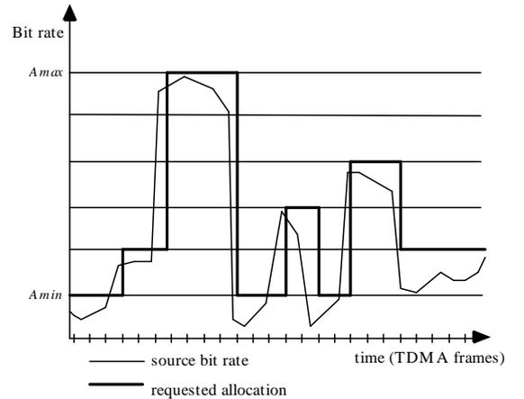
Figure 1. Allocation levels for an input traffic with varying throughput
