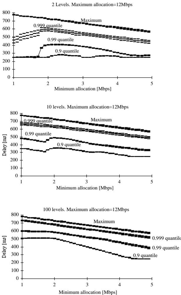
Figure 5. Maximum data delay vs. minimum allocation with 2, 10, 100 allocation levels.
