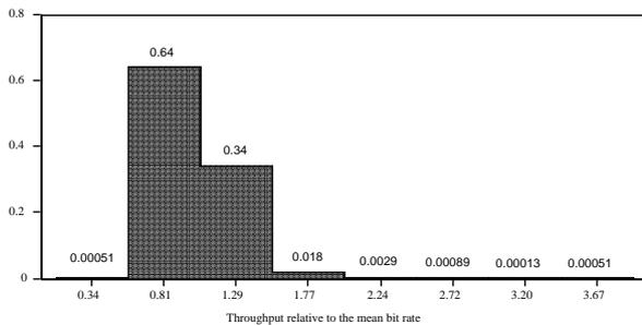
Figure 2. Probability density function of the bit rate produced by the Markov generator
