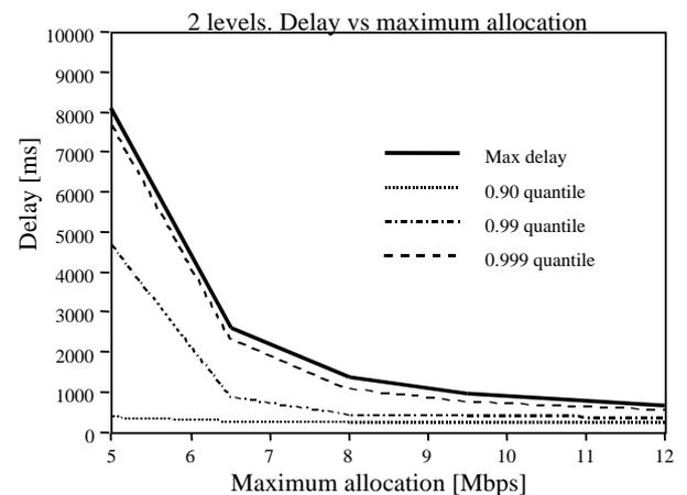
Figure 3. Maximum data delay vs. maximum allocation. Two allocation levels with a minimum allocation equal to 3 Mbps.
