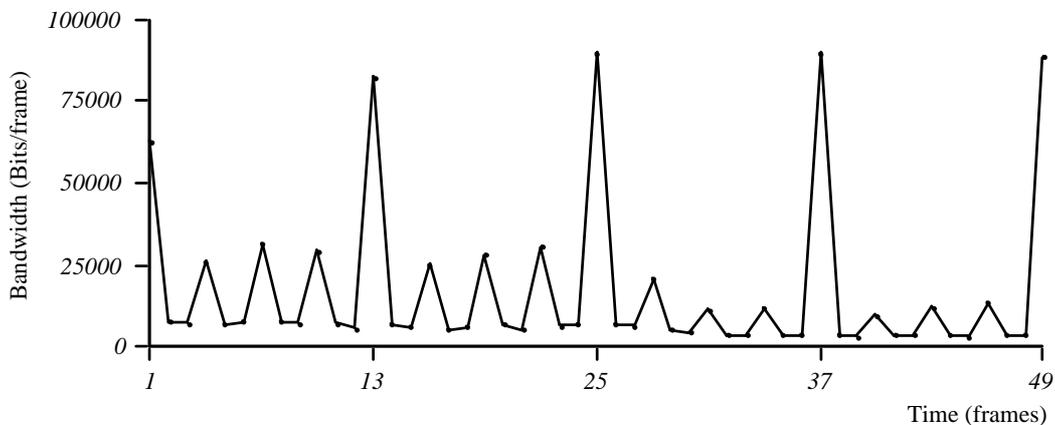
Figure 6. Part of the MPEG-1 coder trace, revealing group length and frame pattern.
