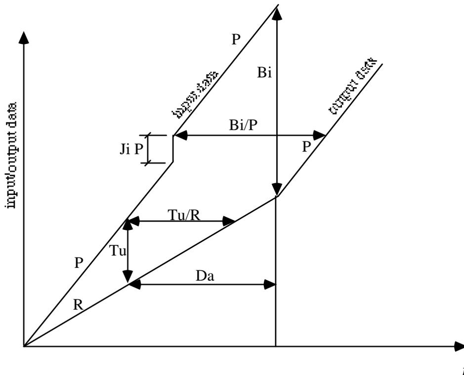
Figure 4. Buffer requirements and queuing times relationships in the transition from allocation  $R$  to allocation  $P$  (worst case).
