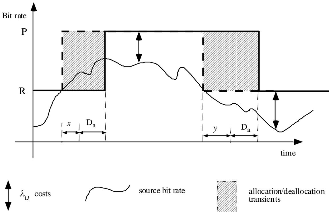
Figure 8. Real-time bandwidth lost due to dynamic allocation.
