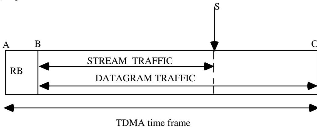
Figure 1. TDMA frame structure in V2L-DA
