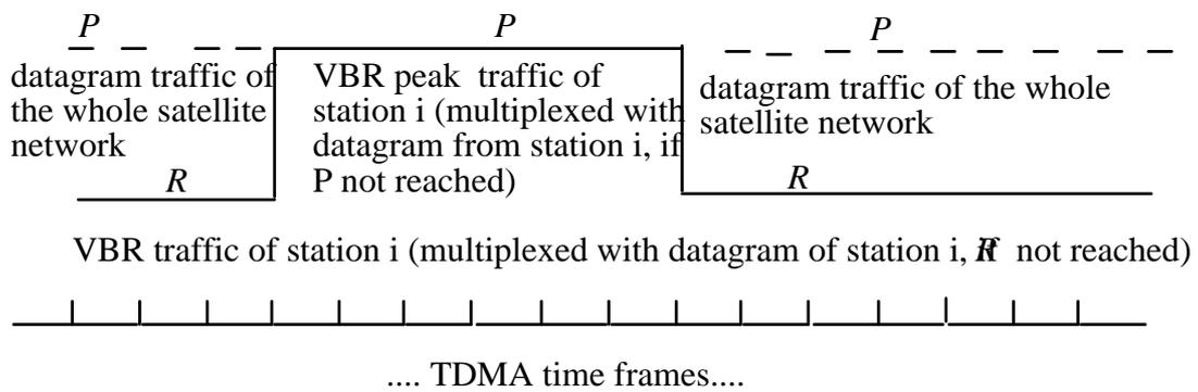
Figure 2. Relationship between the *booked* bandwidth  $P$  (dashed line) and the *allocated* bandwidth, either  $R$  or  $P$  (solid line).
