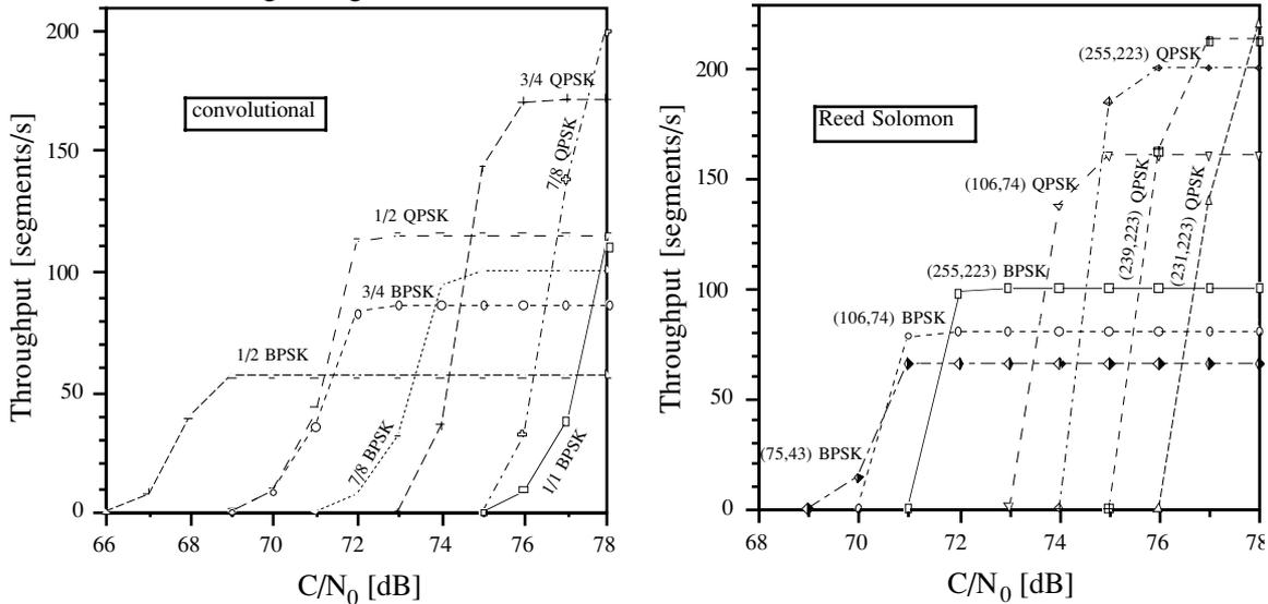
Fig. 2. TCP goodput versus  $C/N_0$  for convolutional (CV) and Reed-Solomon (RS) codes.
