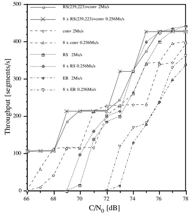
Fig. 4. Goodput envelopments of one TCP connection and the aggregated goodput of 8 TCP connections that share the same amount of bandwidth, versus  $C/N_0$ , for different coding types.
