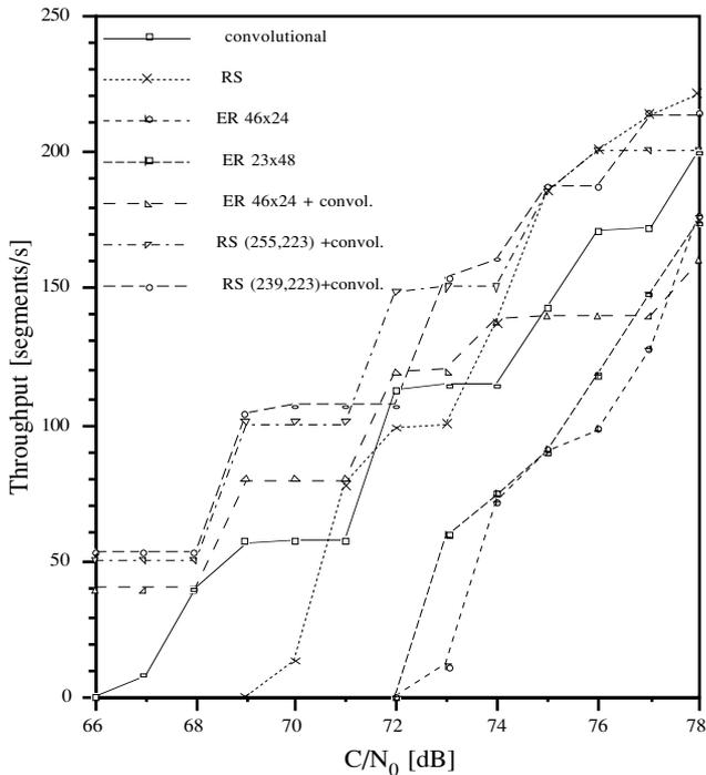
Fig. 3. Maximum goodput versus  $C/N_0$  for different coding types.
