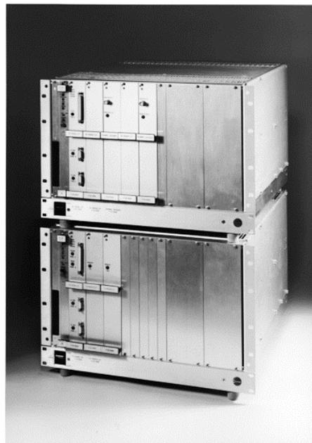
Figure 1. The TDMA controller hardware
