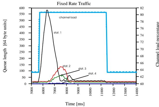
Fig. 25. Queue length versus time when station 1 has a traffic step of 17% of the channel capacity (step duration = 5.5 s).
