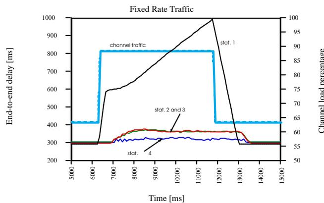
Fig. 23. Single station delay versus time when station 1 has a traffic step of 25% of the channel capacity (step duration = 5.5 s).
