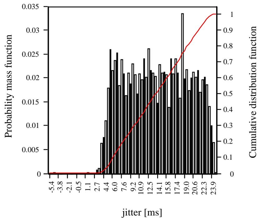
Fig. 12. Jitter distribution for  $\delta = 6$  ms; no bursty data present on the channel; initial jitter span = 6 ms.
