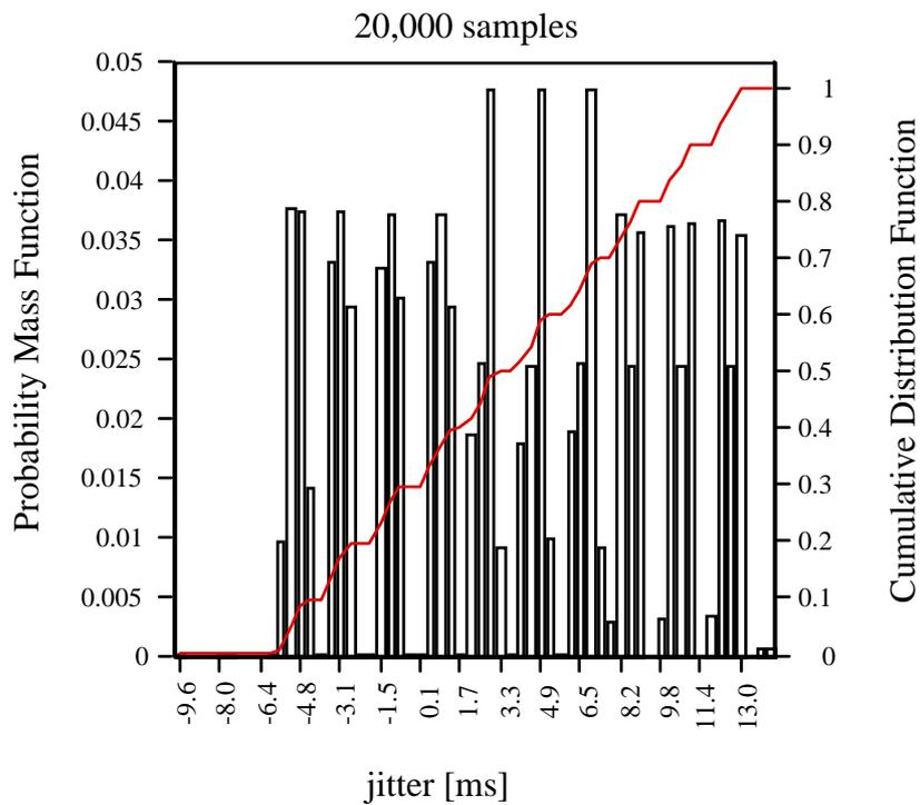
Fig. 11a. Jitter distribution for  $\delta = 6$  ms; no bursty data on the channel; no initial jitter. 20,000 samples.
