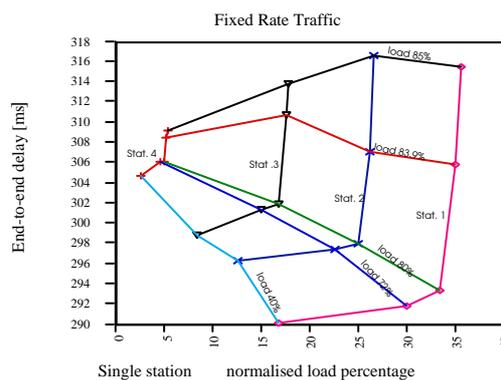
Fig. 18. Single station mean delay versus station load for fixed rate traffic.
