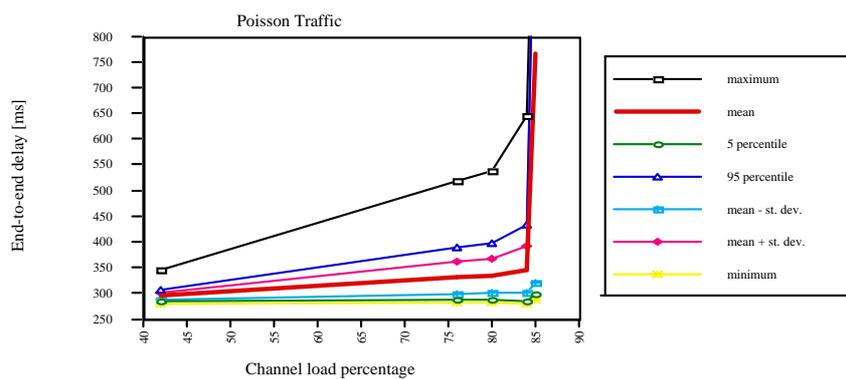
Fig. 21. Channel end-to-end delay statistics versus the channel load for Poisson traffic.
