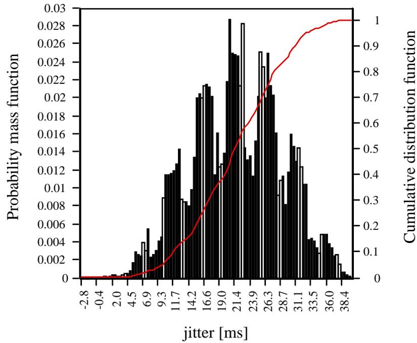
Fig. 8. Jitter distribution for  $\delta = 35$  ms; no bursty data present on the channel; initial jitter span = 24 ms.
