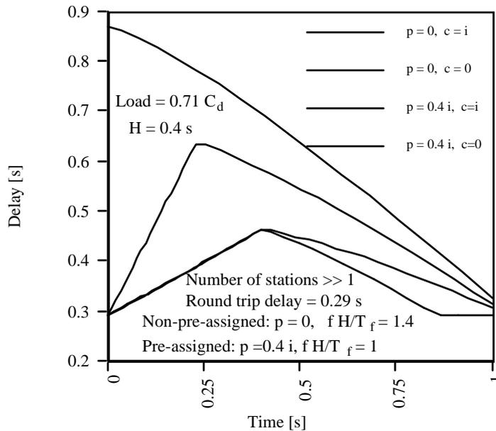
Fig. 4. End-to-end delay versus time during a transient due to a step of traffic at one station. A large number of stations is considered. Pre-assignment and non pre-assignment cases for pre-loaded and for non pre-loaded stations are reported.
