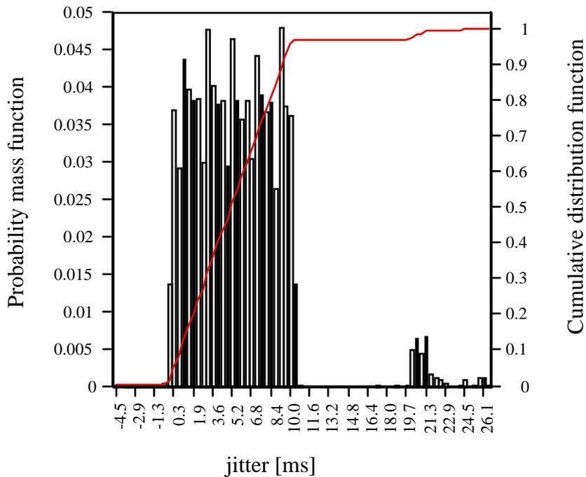
Fig. 9. Jitter distribution for  $\delta = 20$  ms; bursty data present on the channel; no initial jitter.
