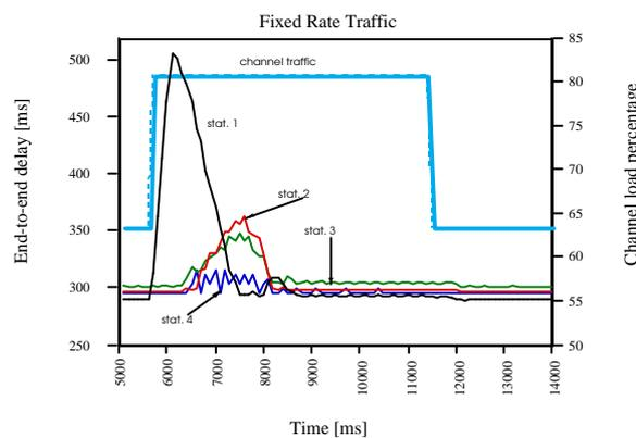
Fig. 24. Single station delay versus time when station 1 has a traffic step of 17% of the channel capacity (step duration = 5.5 s).
