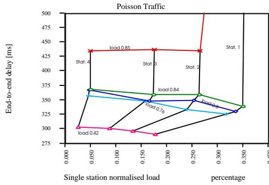
Fig. 19. Single station mean delay versus station load for Poisson traffic.
