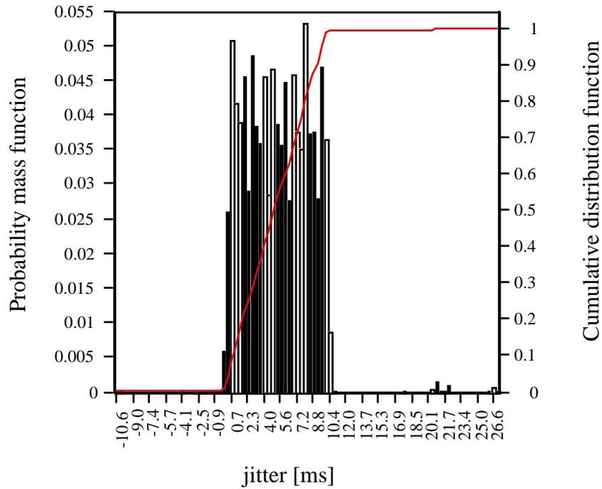
Fig. 10. Jitter distribution for  $\delta = 20$  ms; bursty data present on the channel; initial jitter span = 19 ms.
