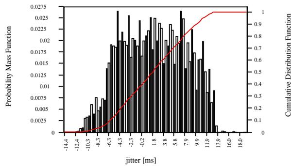
Fig. 14. Jitter distribution for  $\delta = 6$  ms; bursty data present on the channel; initial jitter span = 6 ms.
