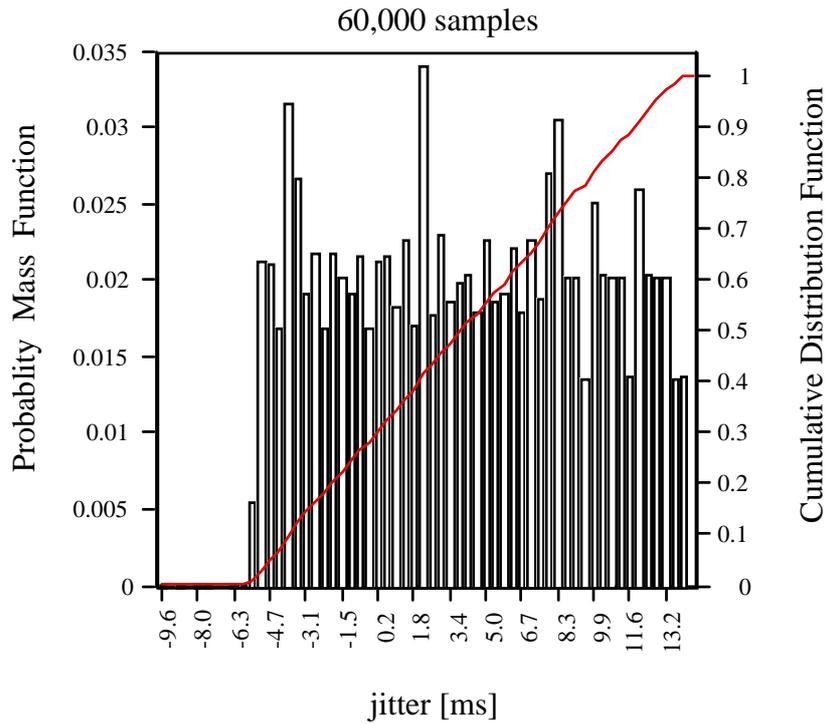
Fig. 11b. Jitter distribution for  $\delta = 6$  ms; no bursty data on the channel; no initial jitter. 60,000 samples.
