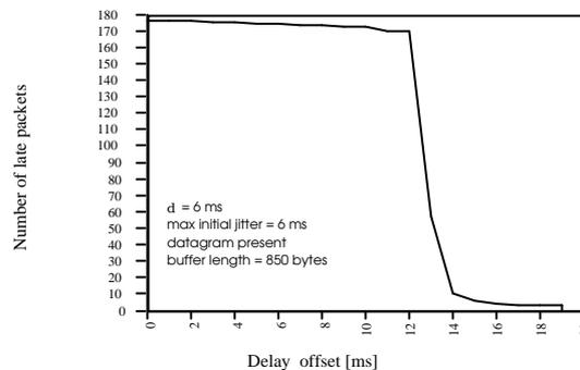
Fig. 17. Late packets versus delay offset;  $\delta = 6$  ms; bursty data present on the channel; initial jitter span = 6 ms.
