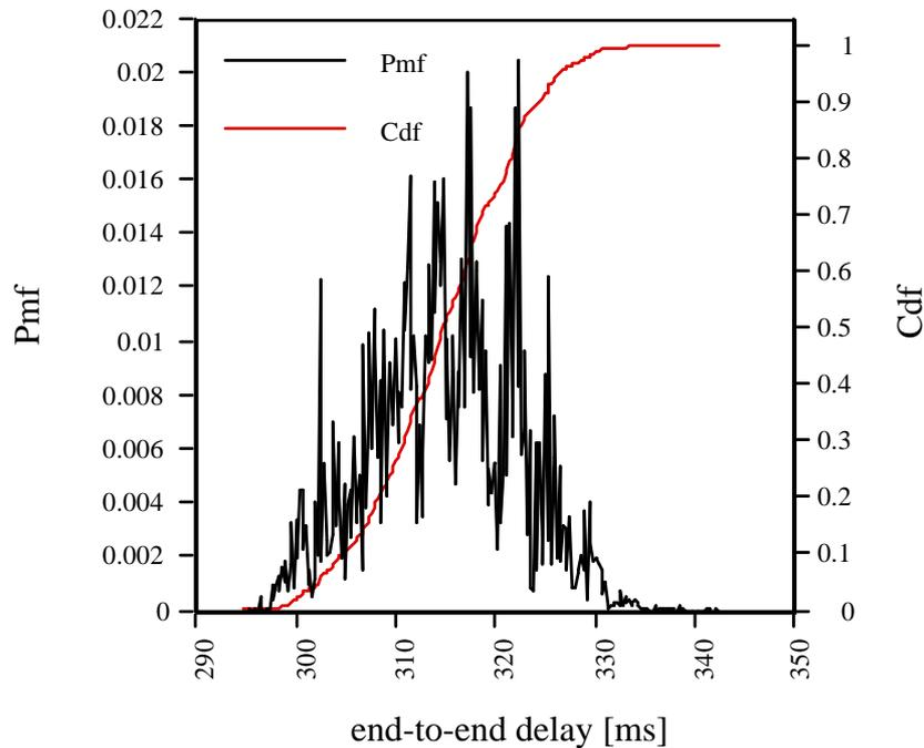
Fig. 22. End-to-end delay distributions: probability mass function and cumulative distribution function. Channel loaded with 85% fixed rate traffic.
