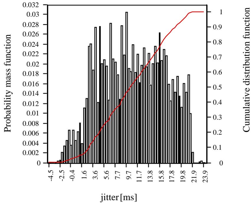
Fig. 13. Jitter distribution for  $\delta = 6$  ms; bursty data present on the channel; no initial jitter.
