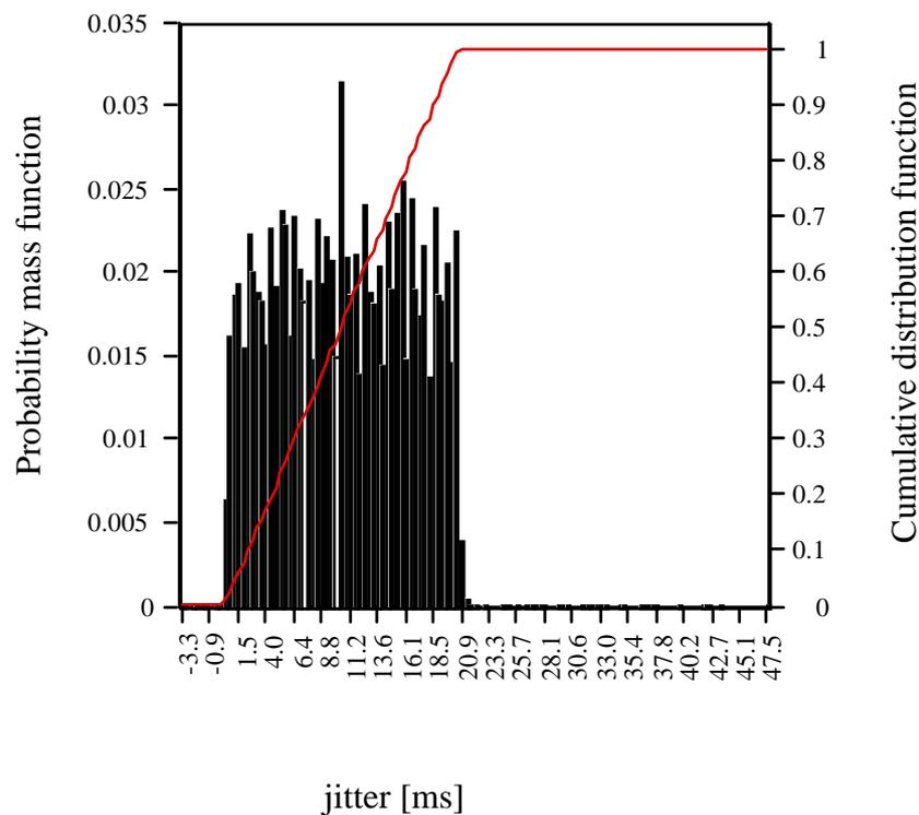
Fig. 5. Jitter distribution for  $\delta = 35$  ms; bursty data present on the channel; no initial jitter.
