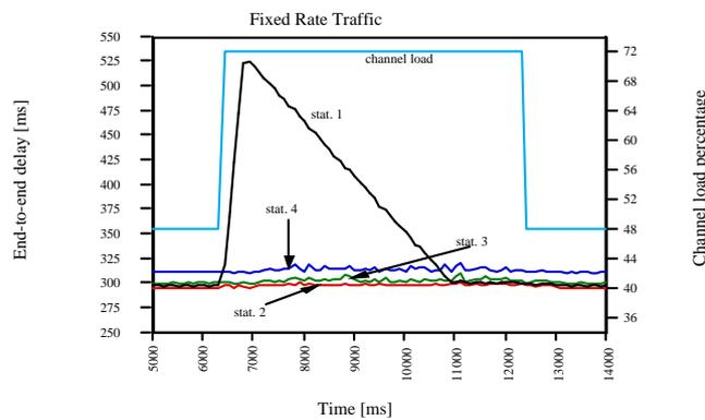
Fig. 26. Single station delay versus time when station 1 has a traffic step of 24% of the channel capacity (step duration = 5.5 s).
