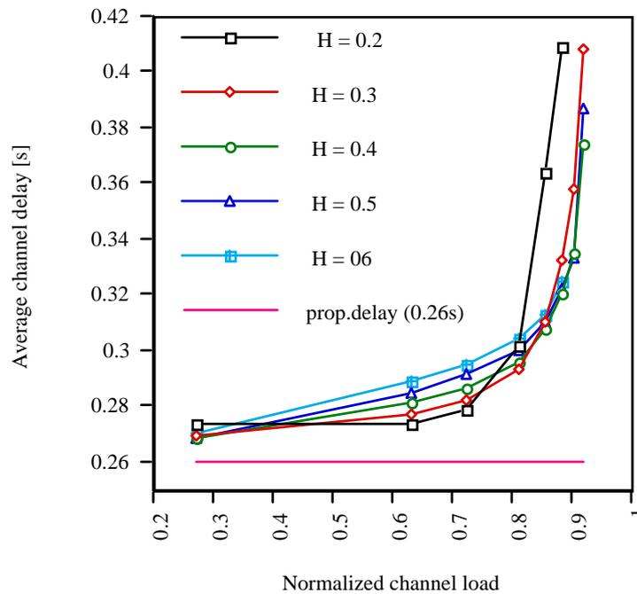
Fig. 2. Average end-to-end delay (10 stations), versus channel load, for various values of  $H$ . The system is loaded with Poisson generators. The channel load includes the packet headers.
