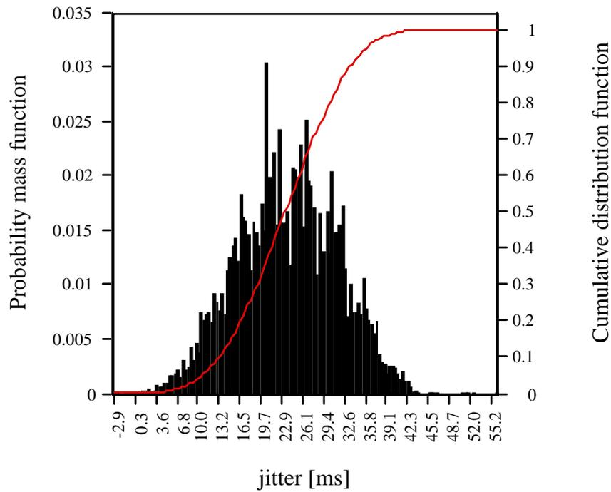
Fig. 6. Jitter distribution for  $\delta = 35$  ms; bursty data present on the channel; initial jitter span = 34 ms.
