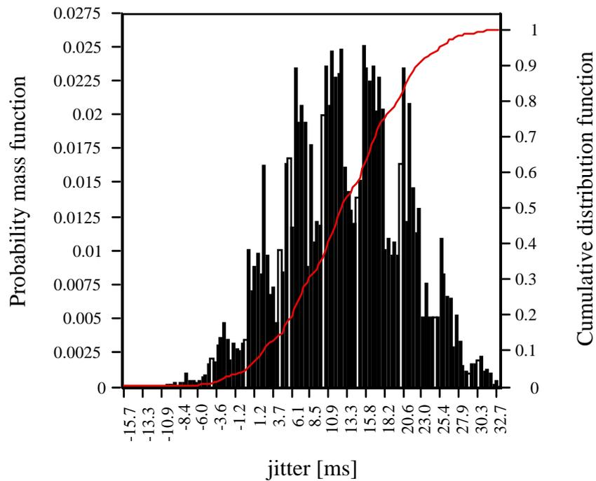
Fig. 7. Jitter distribution for  $\delta = 35$  ms; no bursty data present on the channel; initial jitter span = 34 ms.
