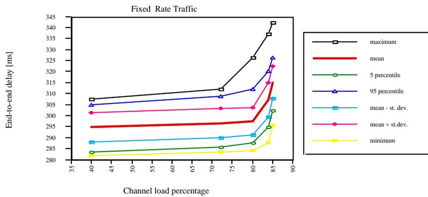
Fig. 20. Channel end-to-end delay statistics versus the channel load for fixed rate traffic.
