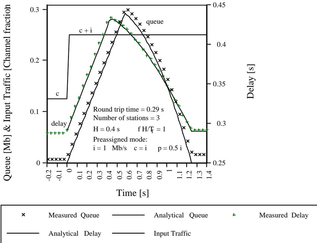
Fig. 3. Queue and delay versus time during a transient due to a 1Mbit/s traffic step at one of the three working stations. Comparison between analytical and experimental results.
