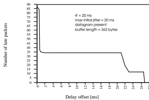
Fig. 16. Late packets versus delay offset;  $\delta = 20$  ms; bursty data present on the channel; initial jitter span = 20 ms.
