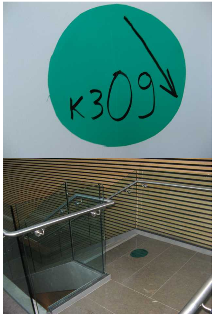
Fig. 1. The reference localization system: when the actor steps over the green mark, he presses the button of the logging application (section III-B).
