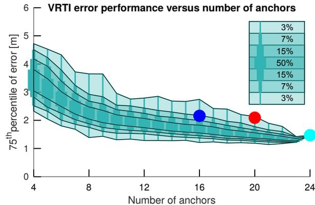
**Figure 3:** Error performance (75<sup>th</sup> percentile of error) for 15890 different anchor configurations. A variable number of anchors is ignored starting from the 24-anchors measurement. The red and blue dots represent the 20- and 16-anchors measurements.
