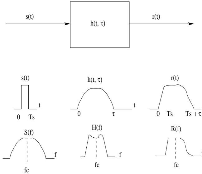
**Fig. 3.9.** Frequency selective fading channel characteristics
