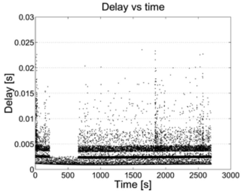
Fig. 2.9. Typical trend of packet delay for the WLAN channel with Retry 7 in 45 minutes of transmission.
