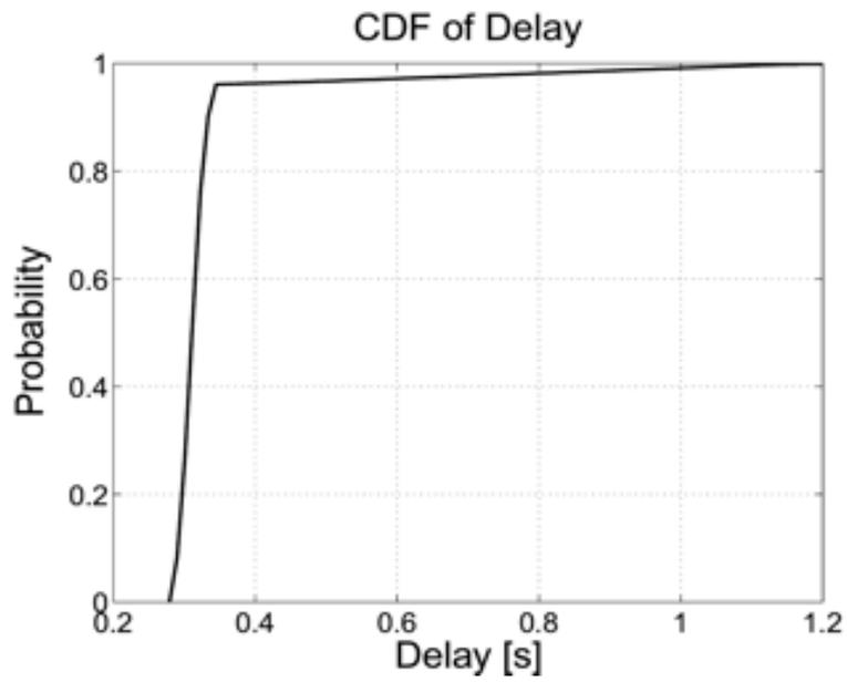
Fig. 2.3. CDF of packet delay for data in 2.2.
