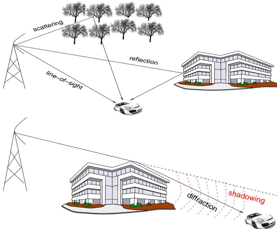
Fig. 3.1. A typical scenario of mobile radio communications
