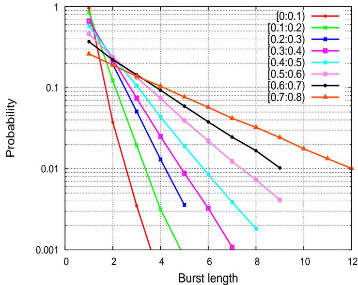
Fig. 7.5. Probability mass function of burst lengths.
