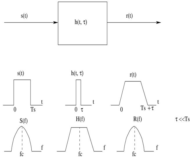
**Fig. 3.7.** Flat-fading channel characteristics
