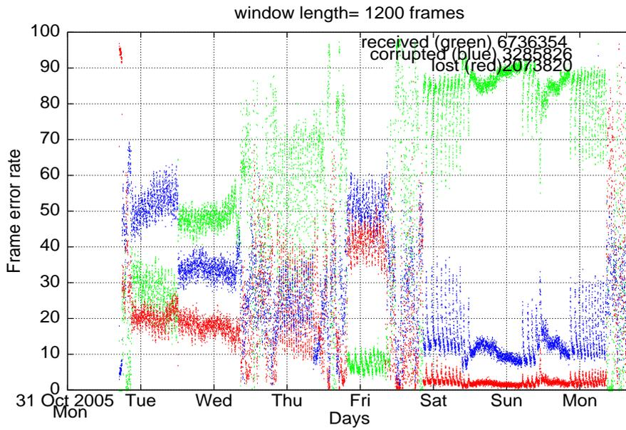
Fig. 8.2. Average of received, lost and corrupted frames during the first week.
