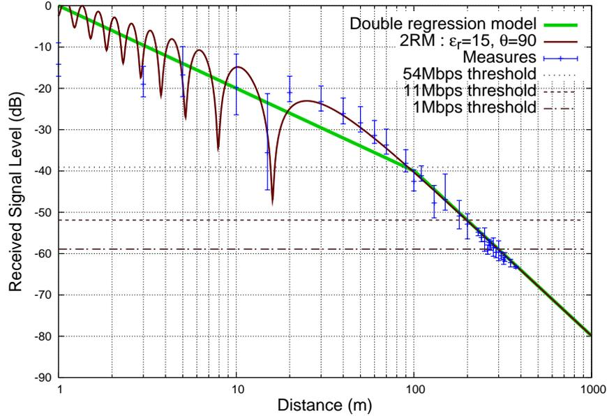
**Fig. 7.2.** Measured signal level, double regression model and two-ray model with sensitivity thresholds for  $\Delta L = 0$ . Error bars indicate 0.05, 0.50 and 0.95 quantiles of observed values.
