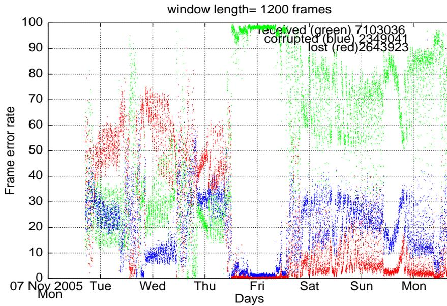
Fig. 8.3. Average of received, lost and corrupted frames during the second week.
