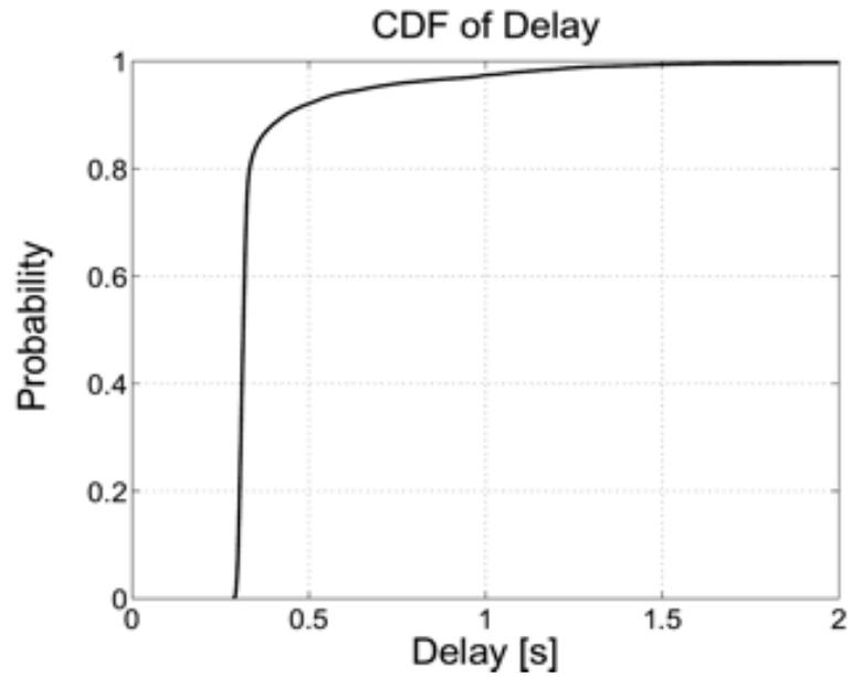
Fig. 2.15. CDF of packet delay for data in Fig. 2.14.
