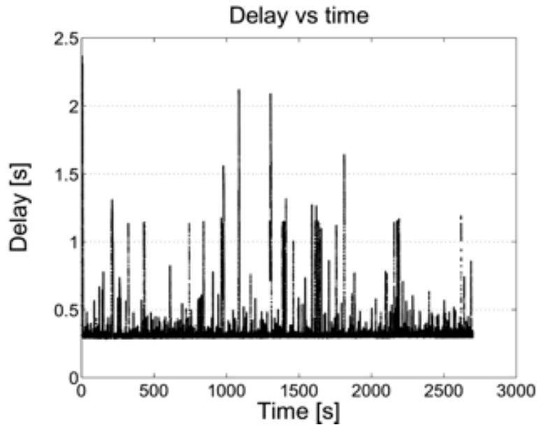
Fig. 2.14. Packet delay for the full path in 45 minutes of real video streaming.
