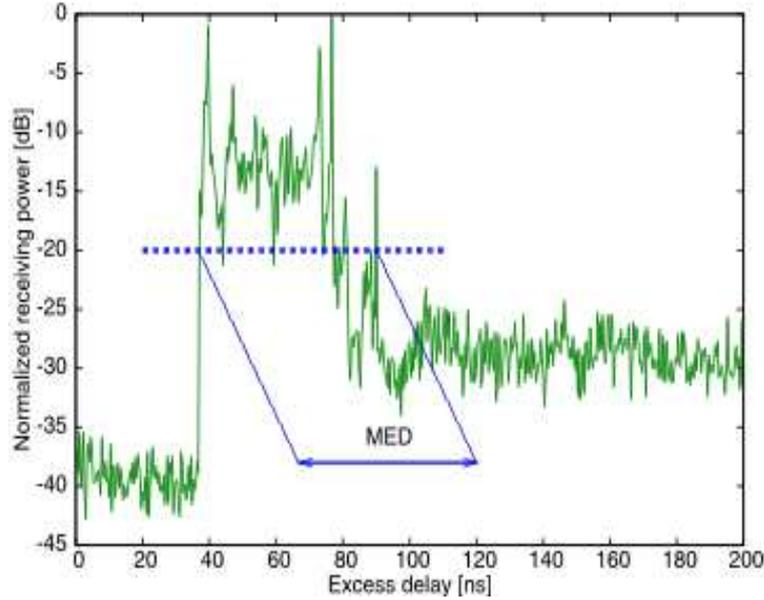
Fig. 3.13. Maximum excess delay
