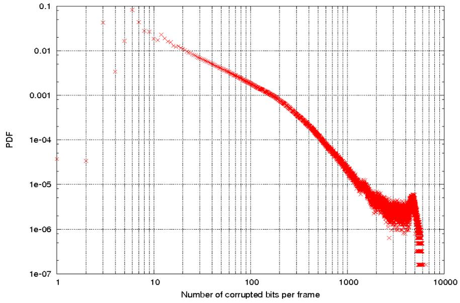
Fig. 8.9. Probability mass function of number of errored bits per frame
