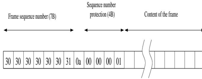
**Fig. 6.2.** Transmitted frame.
