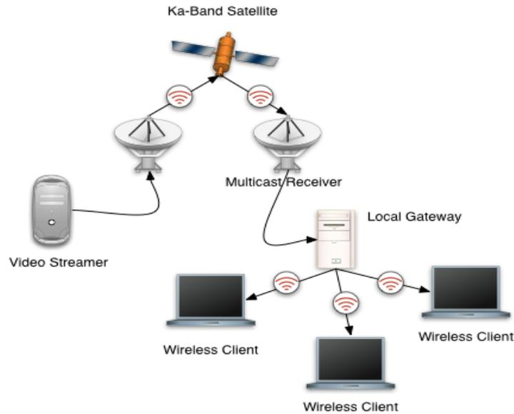
Fig. 2.18. The test-bed network topology.
