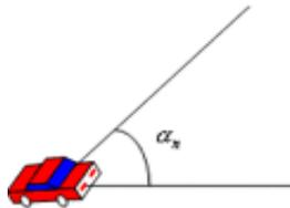
**Fig. 3.2.** Angle of arrival of the  $n^{th}$  incident wave
