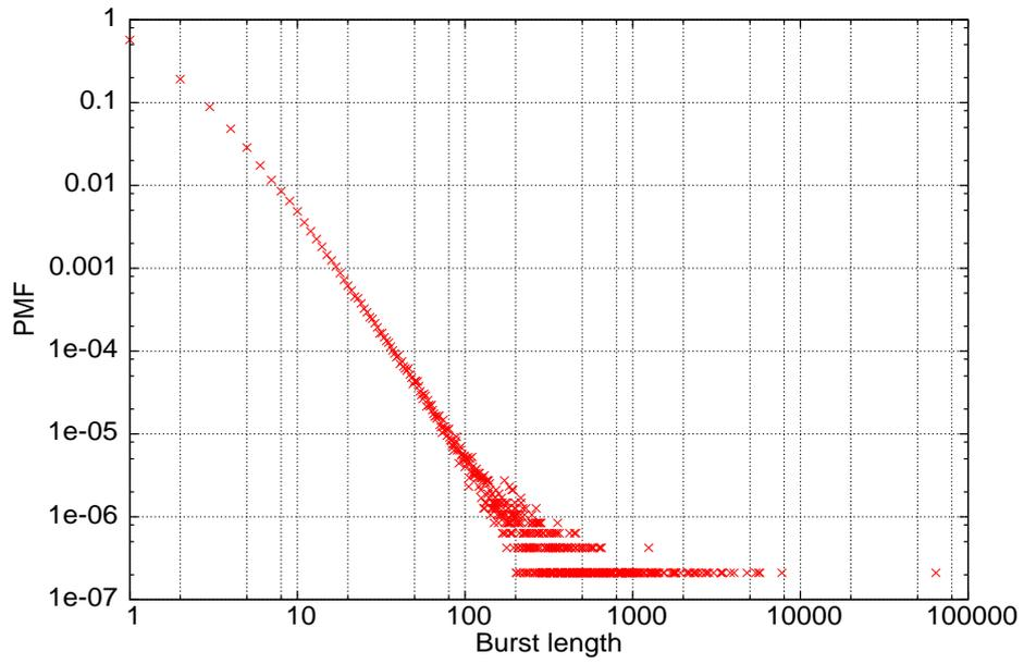
Fig. 8.5. Probability mass function of burst length at frame level.
