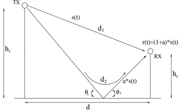
**Fig. 4.1.** 2-ray ground reflection model.
